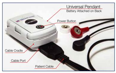
Clip the provided lanyard accessory onto the loop at the top of the Cable Cradle to wear it around your neck. Alternatively, you may carry it in your pocket but be careful that the Patient Cable remains firmly connected.
