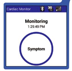
**6.** When the monitor has recognized your heart's electrical signal, the waveform will disappear and the Handset screen will display Monitoring and a Symptom button.
